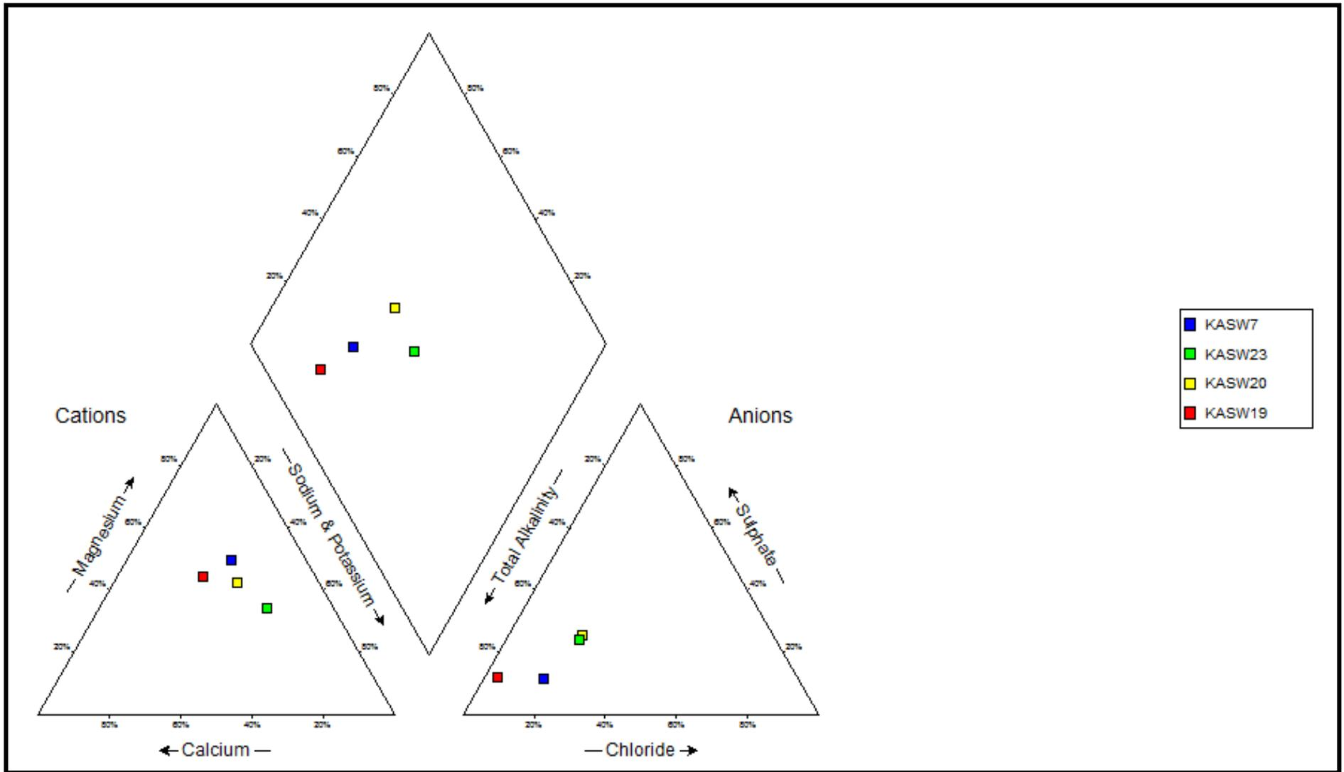
Figure 19: Piper diagram of the surface water samples
