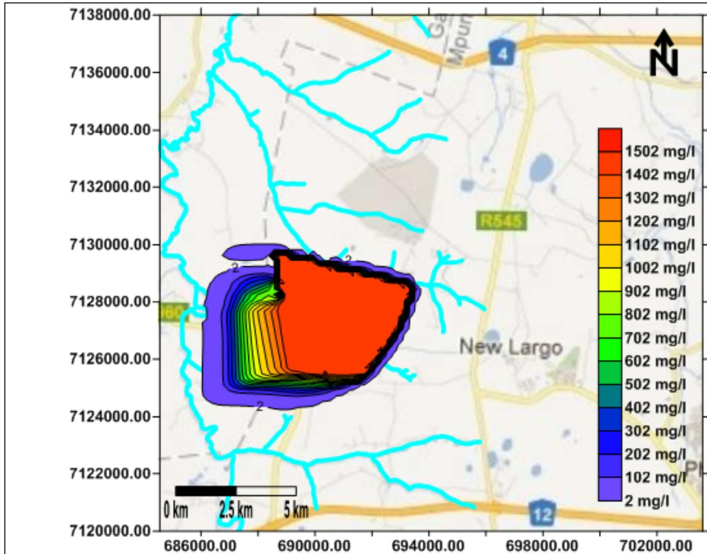
Simulated contamination plume from site A ash dam (non lined) during operation phase (60 years)
