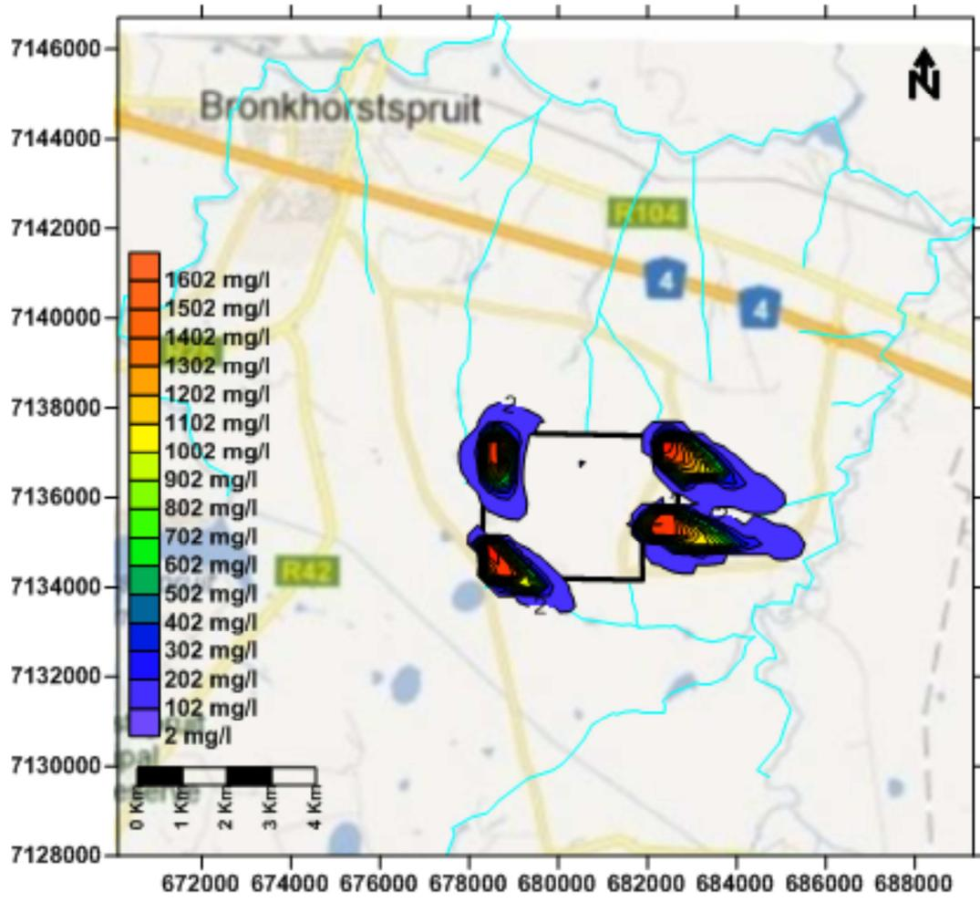
Simulated contamination plume from site B ash dam during operation phase (60 years)
