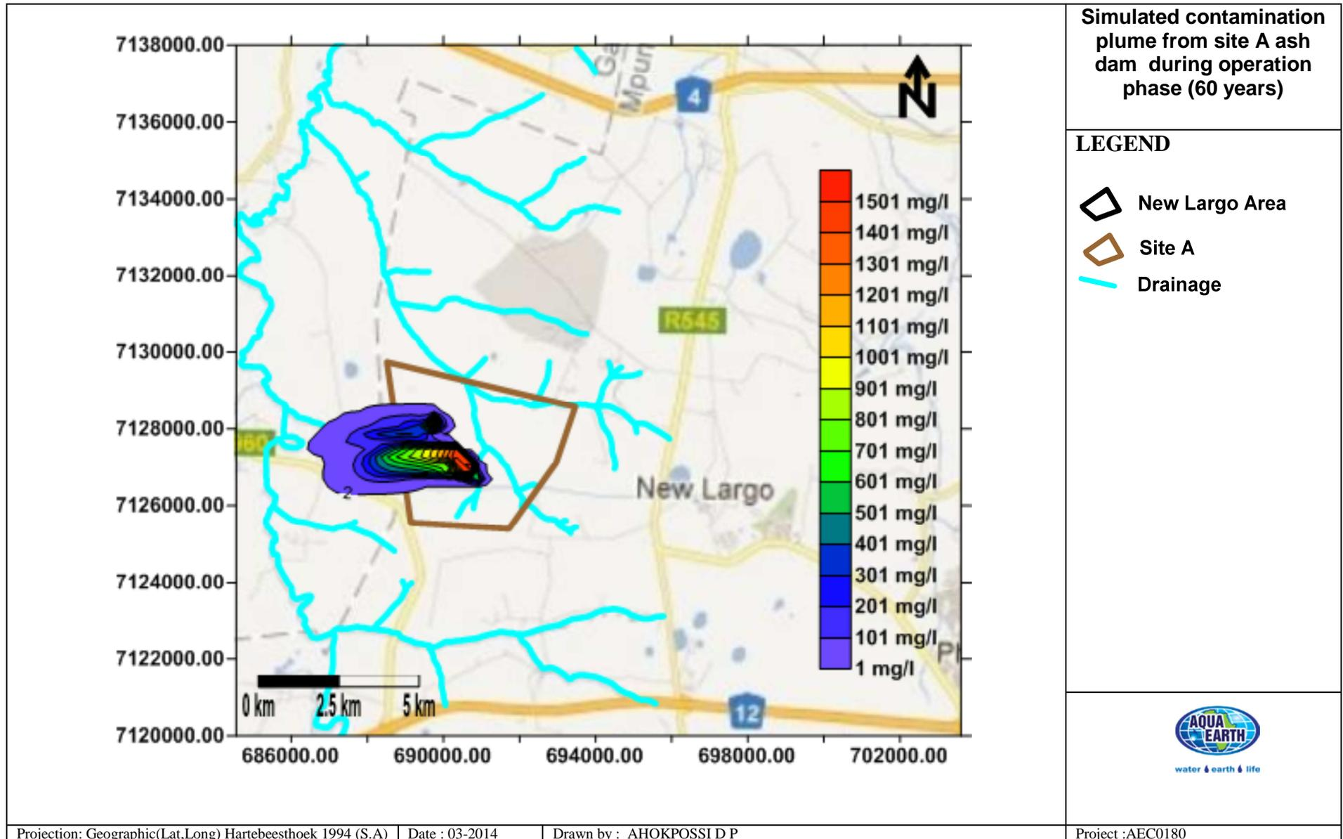
**Figure 59: Contamination plume from Alternative A ADF (2% leakage of lining system) during operation-construction phase (60 years)**
