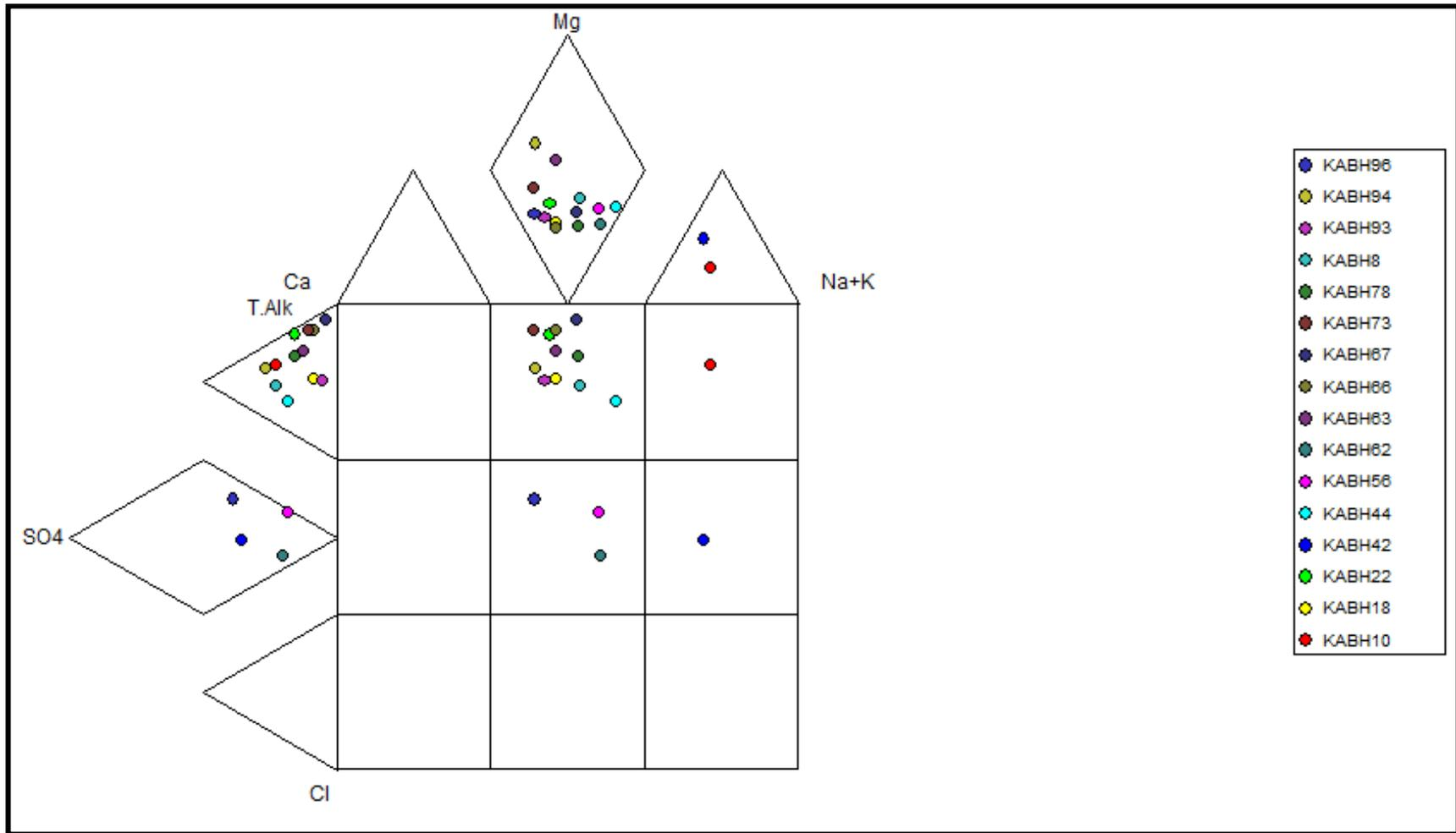
Figure 18 : Expanded Durov Diagram of the groundwater samples
