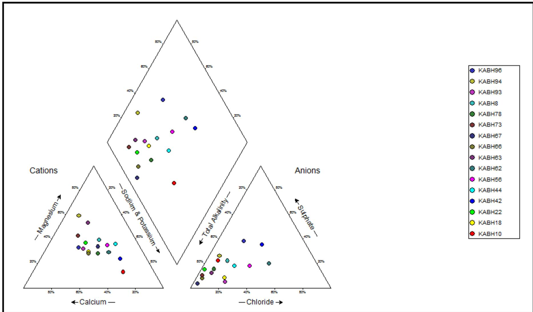
Figure 17: Piper diagram of the groundwater samples
