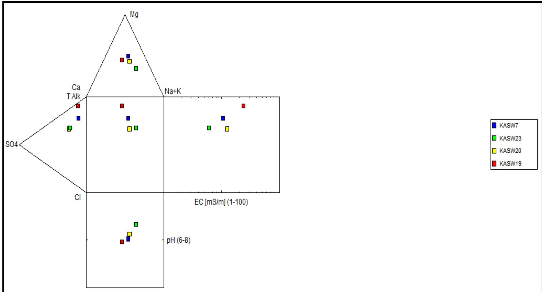
Figure 20: Expanded Durov diagram of the groundwater samples.
