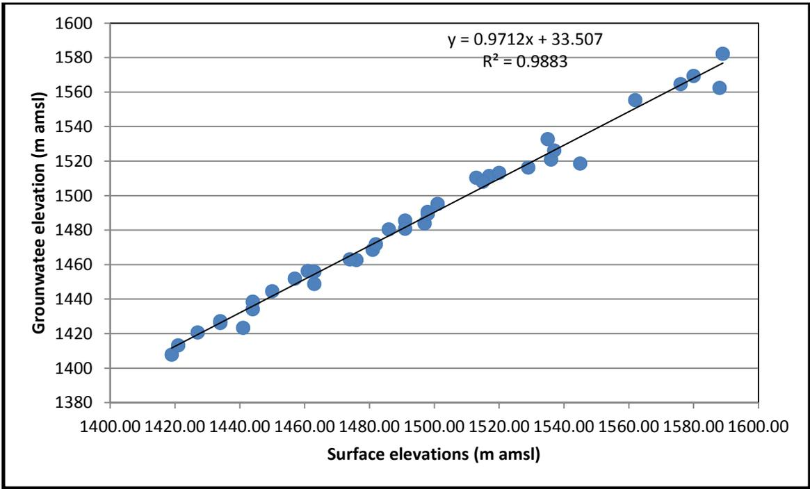
**Figure 11: Surface water elevations and Groundwater elevations correlation**
